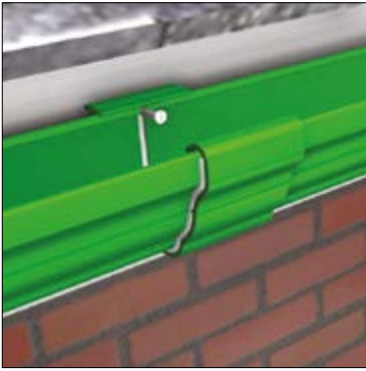
9. Anchor union to fascia board using Alutec 32mm x No. 10 screw, code SC202 or Alutec 15mm x No. 10 countersunk screw, code SC203 if fixing to Alutec aluminium composite fascia. Ensure a 3-4mm expansion gap is left.
